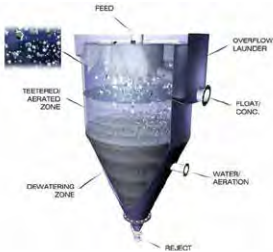
FIGURE 3 Simplified diagram of the HydroFloat® cell
